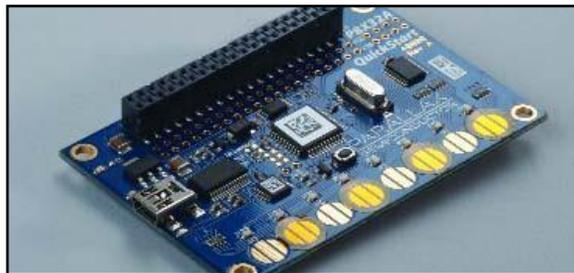
***PCB with labels and tape dots, which can cause ESD when peeled off.***
