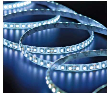
Flexible LED Array With Highly Reflective White Substrate
